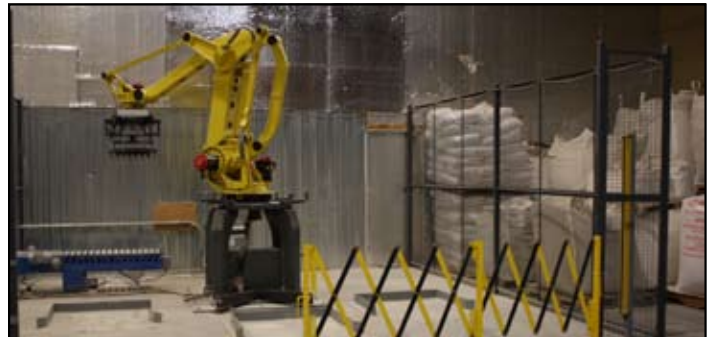
Ralco Nutrition invested in a robot to automate the process of palletizing 50# bags of additives.
